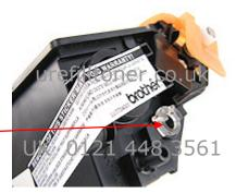
19) Put refilled and loaded cartridge into printer and allow it to initialise. The machine is ready to print again.
